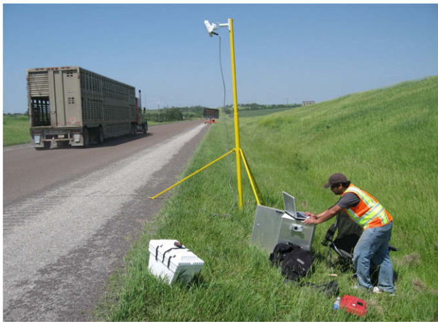
Fig. 3. PCMS and setup of the speed sensor system.
