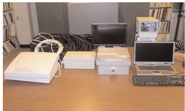
FIGURE 5 Major components of wireless real-time productivity measurement system.
