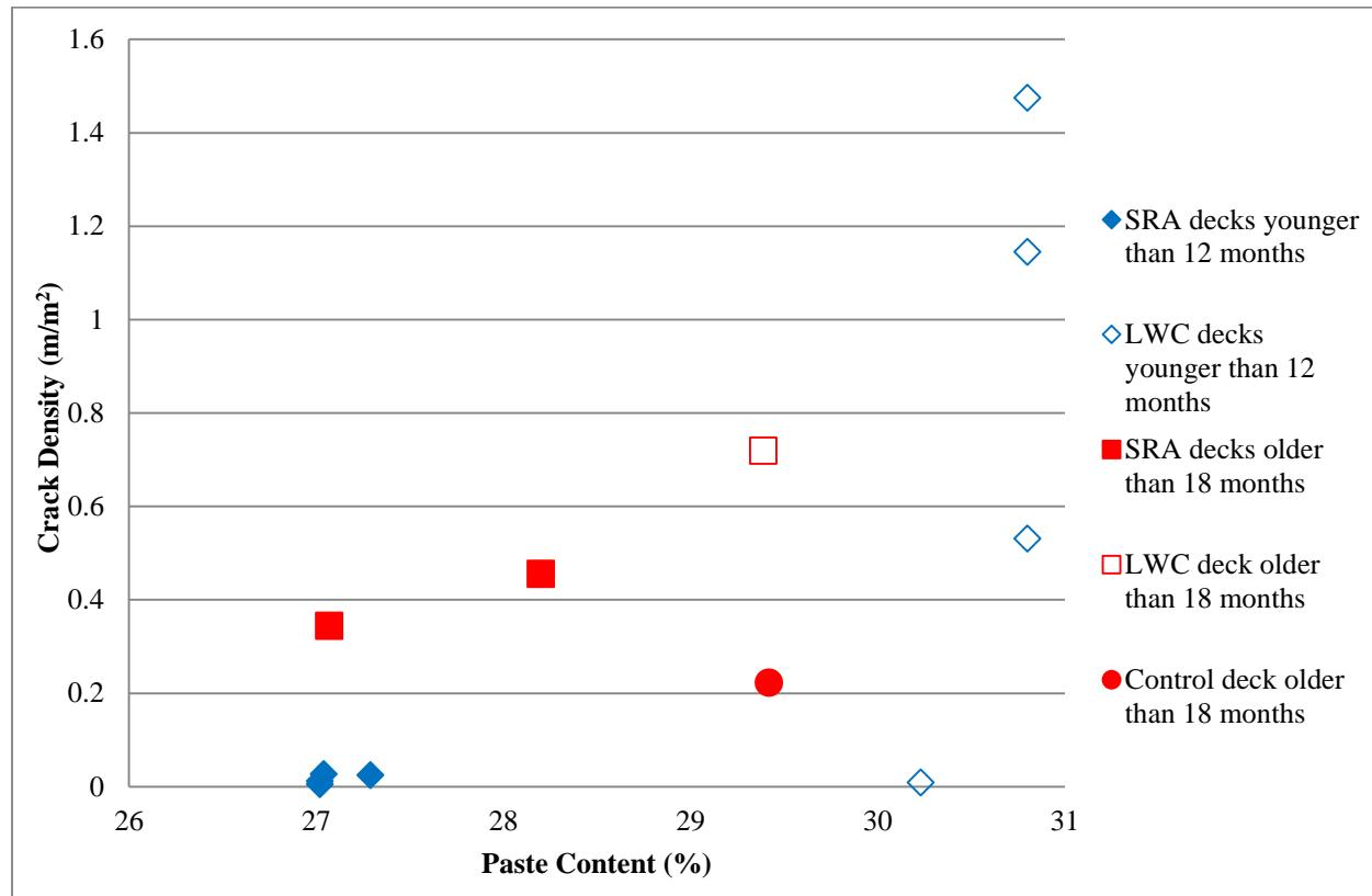
**Figure 14: Crack density versus paste content**
