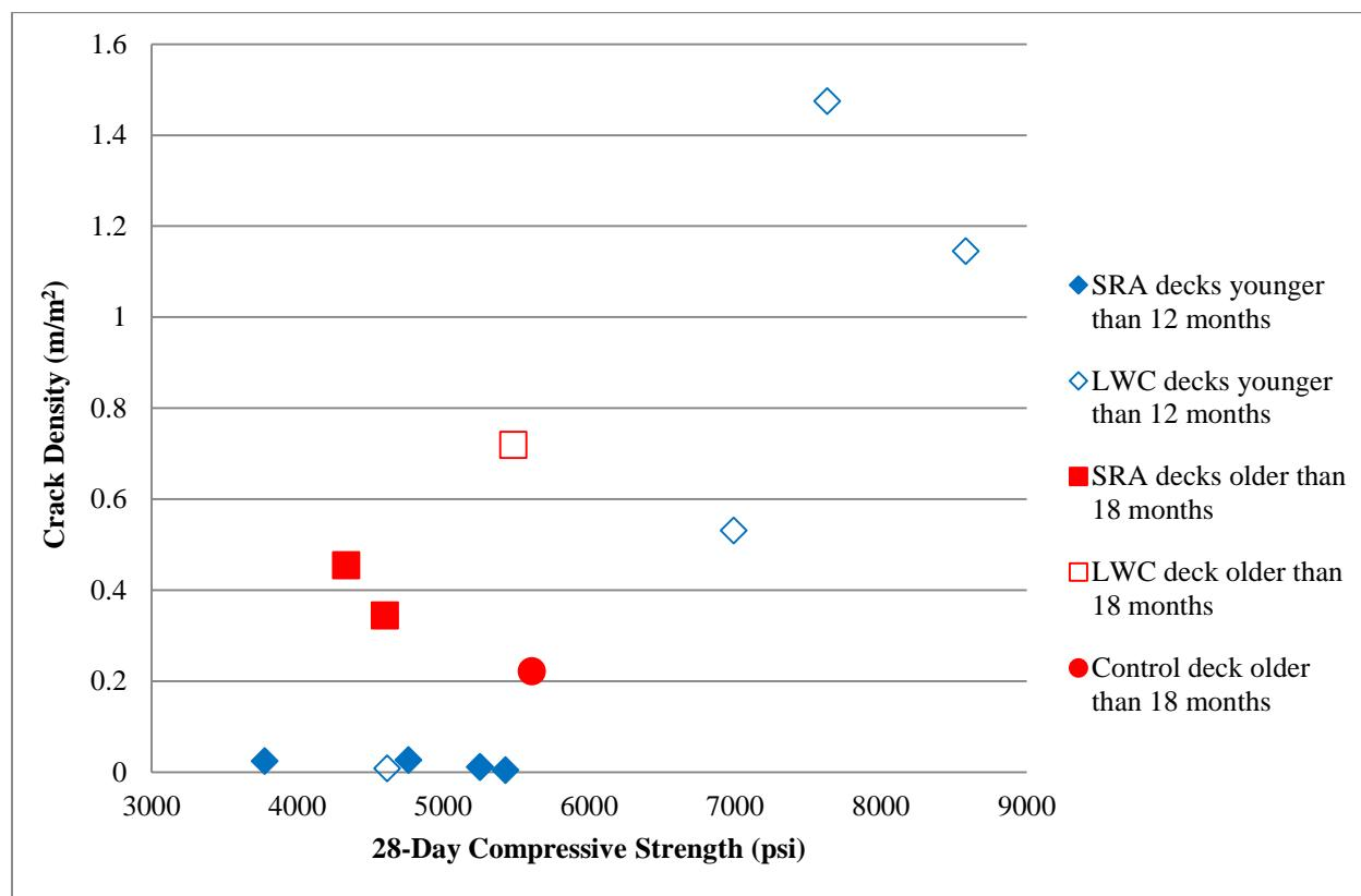
**Figure 15: Crack density versus the 28-day compressive strength of the concrete**
