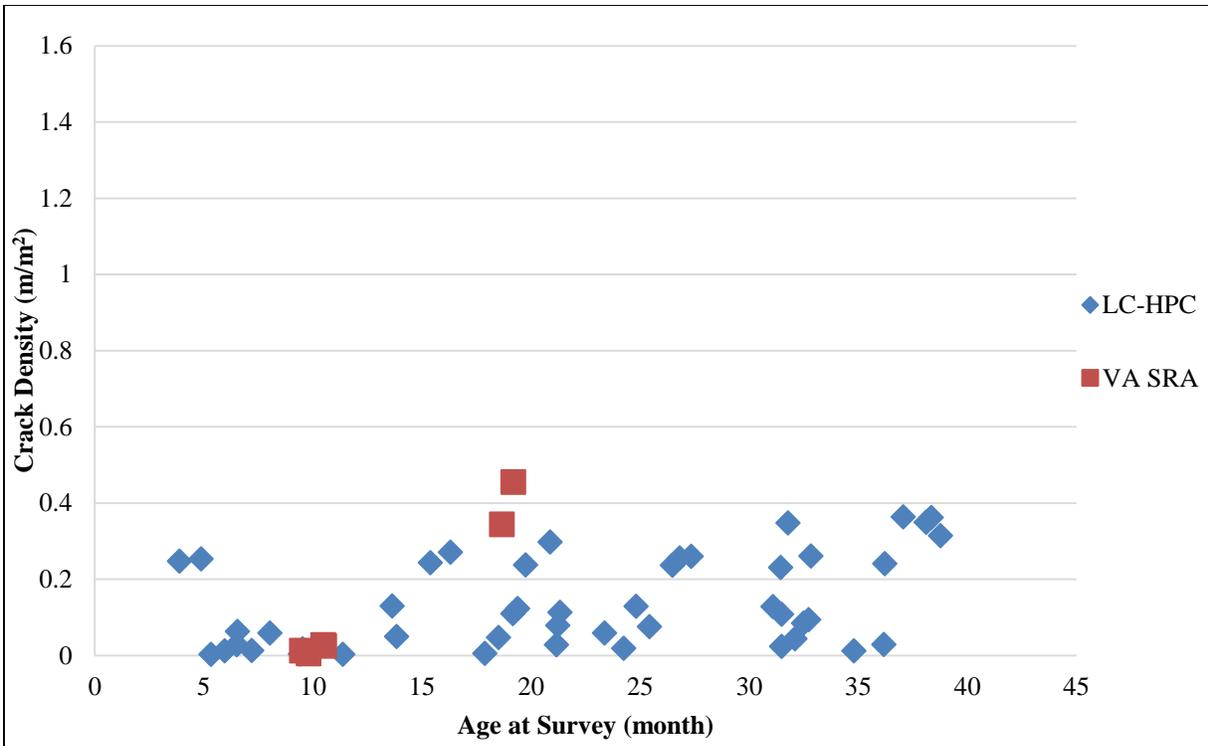
**Figure 11: Crack densities of LC-HPC decks and SRA decks versus bridge age**
