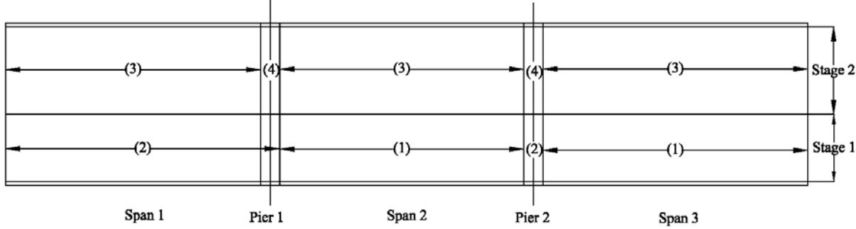
**Figure 9A: Construction Sequence of VA-9**
