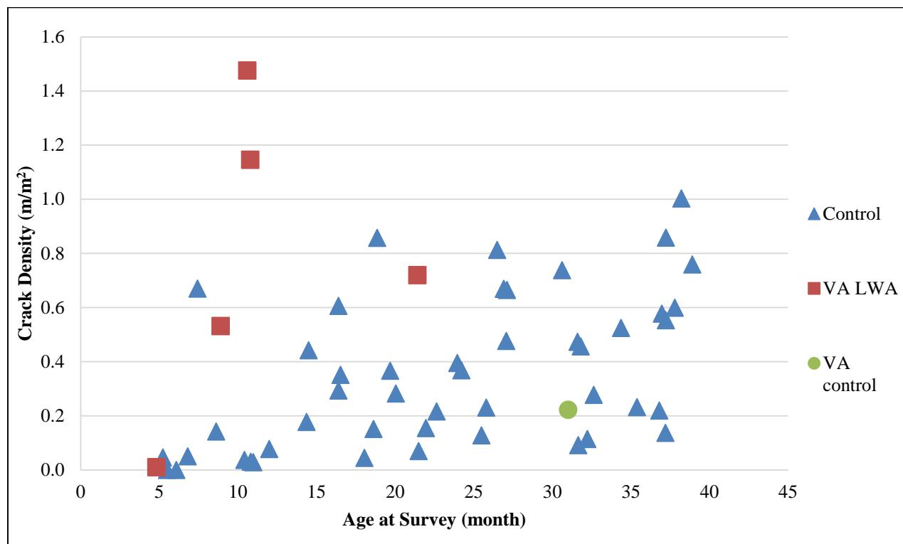
**Figure 12: Crack densities of Virginia bridge decks using lightweight aggregate and control decks versus deck age**
