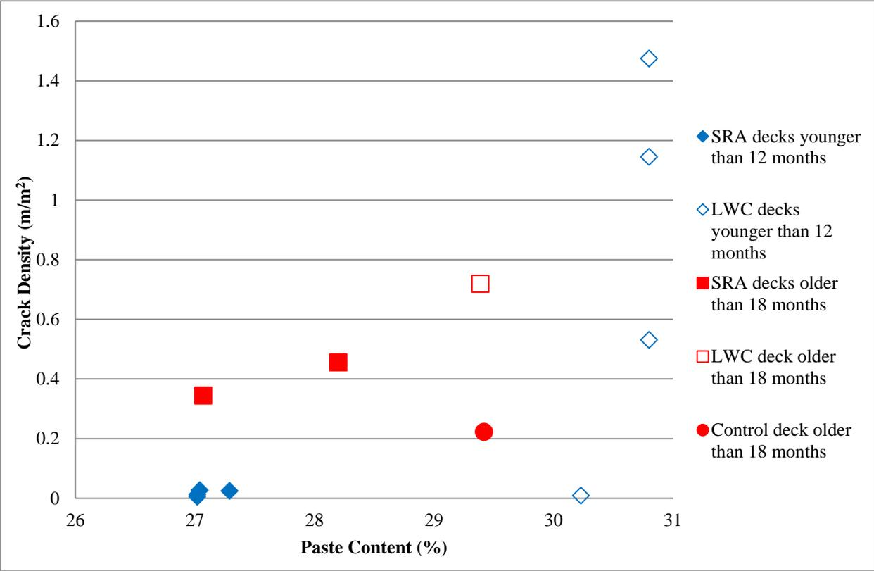
**Figure 14: Crack density versus paste content**
