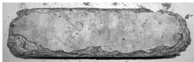
Fig. 10—Specimen subjected to 10 weeks of exposure to 6.04 molal ion concentration solution of MgCl<sub>2</sub>.
