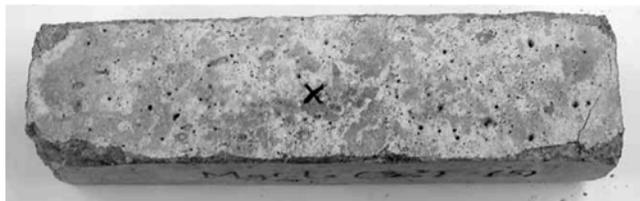
Fig. 6—Specimen subjected to 80 weeks of exposure to 1.06 molal ion concentration solution of MgCl<sub>2</sub>.
