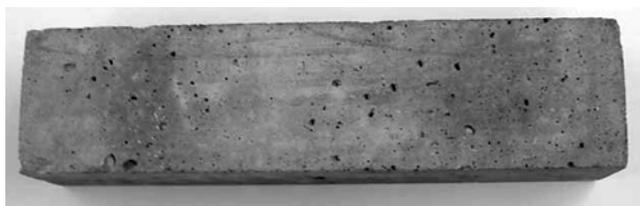
Fig. 5—Specimen subjected to 95 weeks of exposure to 1.06 molal ion concentration solution of CaCl<sub>2</sub>.
