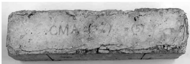
Fig. 7—Specimen subjected to 95 weeks of exposure to 1.06 molal ion concentration solution of CMA.
