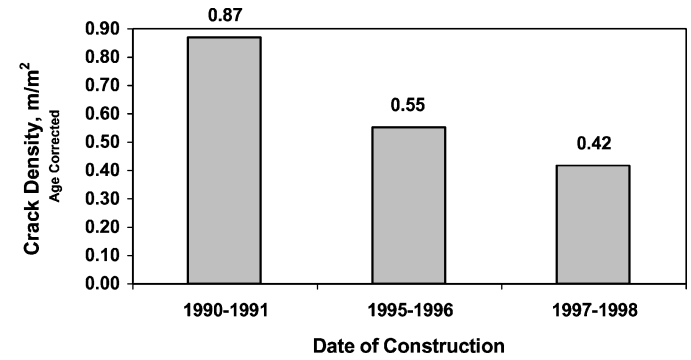
FIG. 15—Mean crack density of entire bridge deck corrected to an age of 78 months versus date of construction for conventional overlay bridge decks.
