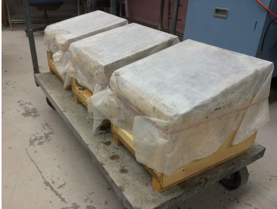
Figure 2.3: Settlement cracking specimens covered with sloped Plexiglas and plastic sheeting.
