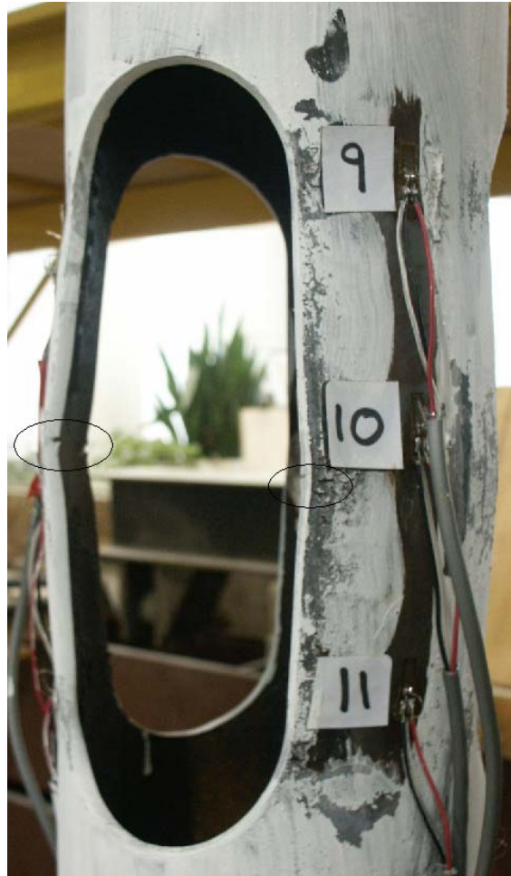
FIG. I1 – FATIGUE FAILURE, LOAD STEP #12, FIRST CYCLE.
