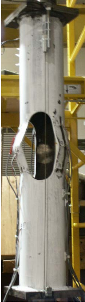
FIG. F2 - PEAK DEFORMATION UNDER COMPRESSION LOAD; LOAD STEP #9 LAST CYCLE.
