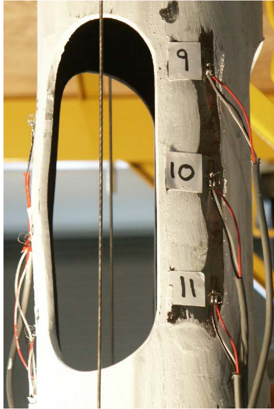
FIG. B3 – BUCKLING DEFORMATION; LOAD STEP #2 LAST CYCLE.
