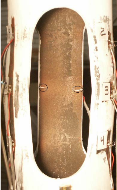
FIG. I3 – FATIGUE FAILURE FROM INSIDE, LOAD STEP #12, FIRST CYCLE.
