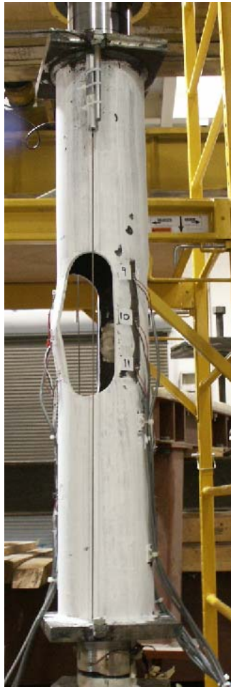
FIG. C1 – BUCKLING DEFORMATION; LOAD STEP #4 LAST CYCLE.
