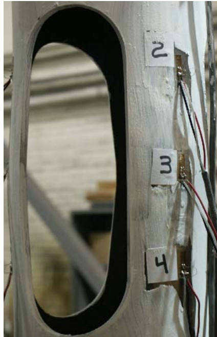
FIG. D1 – INITIAL BUCKLING DEFORMATIONS AT OTHER TWO ARMS LOAD STEP #6.
