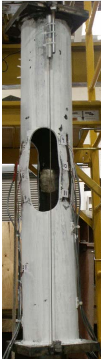
FIG. G1 - PEAK DEFORMATION UNDER TENSION LOAD; LOAD STEP #10 LAST CYCLE.
