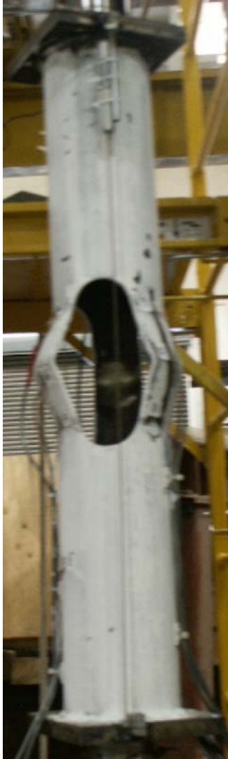
FIG. H2 - PEAK DEFORMATION UNDER COMPRESSION LOAD; LOAD STEP #11 LAST CYCLE.
