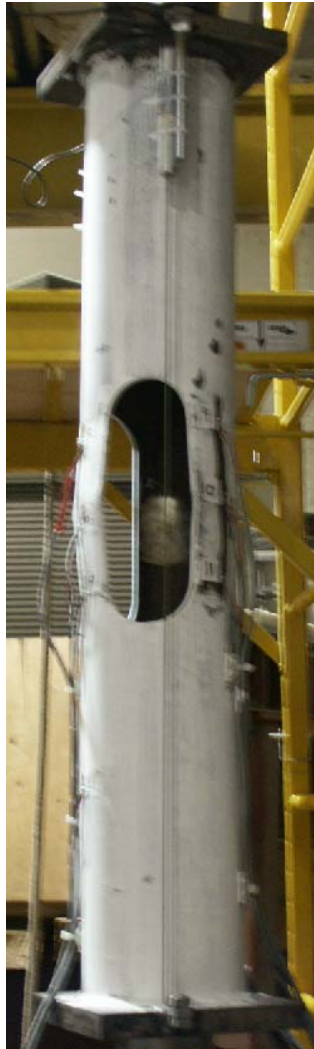
FIG. F1 - PEAK DEFORMATION UNDER TENSION LOAD; LOAD STEP #9 LAST CYCLE.
