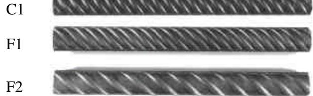
Fig. 8—ASTM A 615 No. 8 rolled bar deformation patterns.
