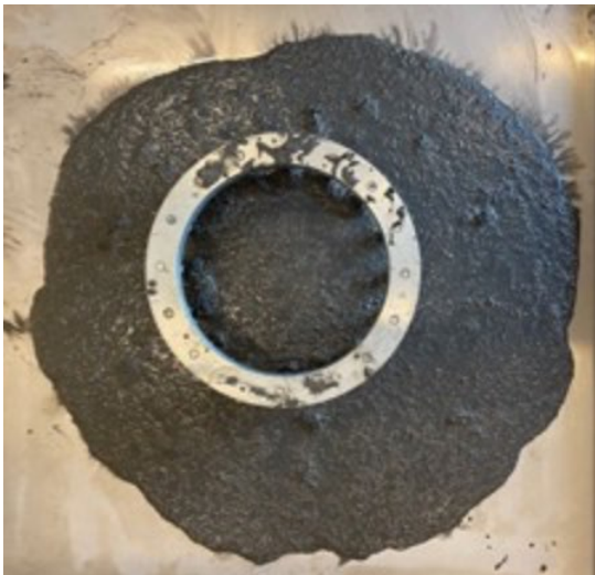
Figure 4.1: J-ring Test of Batch B15–LWA15%
