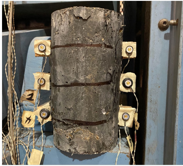
Figure 3.8: Marker Placement on Cylinder
