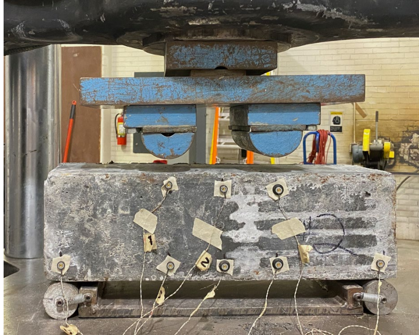
Figure 3.12: Beam Specimen with Eight Markers
