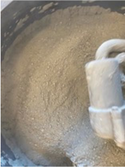
Figure 3.4: Mixture after Adding Cement
