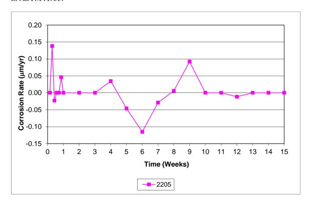
**Figure 5:** Average corrosion rates (μm/yr) for 2205 stainless steel.
