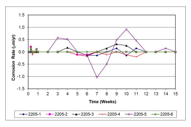
Figure 3: Individual corrosion rates ( $\mu$ m/yr) for 2205 stainless steel.
