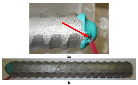
**Figure 4:** (a) Corrosion electrical connection of specimens 2205-5 after testing (b)Specimen 2205-5 after testing
