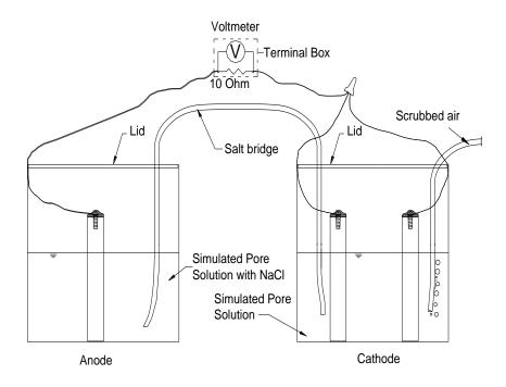
Figure 2: Rapid Macrocell Test Setup
