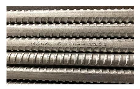
Figure 1: 2205 reinforcing steel evaluated in this report.
