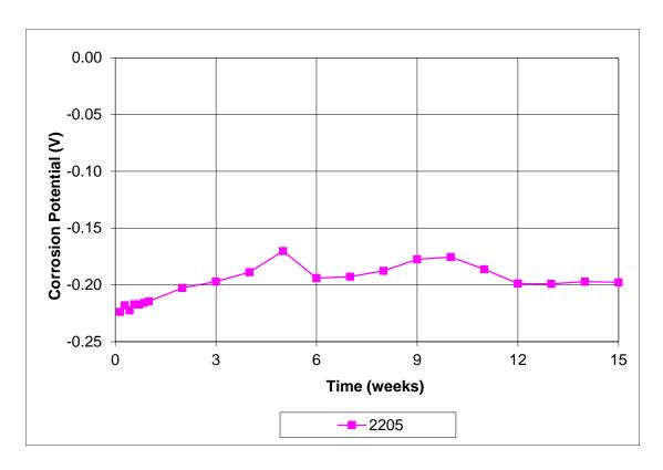
Figure 5: Average corrosion potential (vs. CSE) for 2205 stainless steel.
