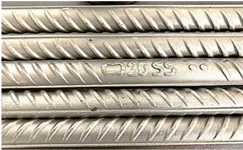
Figure 1: 2304 reinforcing steel evaluated in this report.
