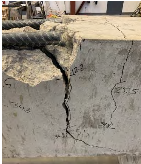
Figure 4.6: Unconfined lap splice failure (14-a)
