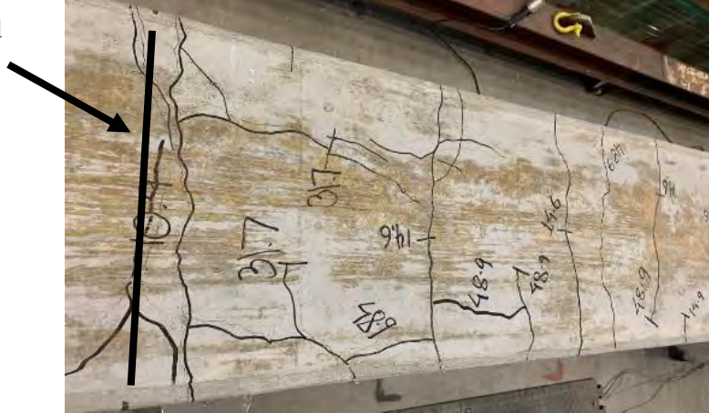
Figure 4.5: Longitudinal splitting cracks (14-f)
