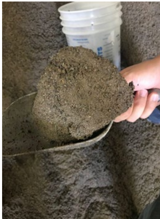
Figure 4.8: A dense clump of LWA observed in the stockpile for MN-IC-LC-HPC-5
