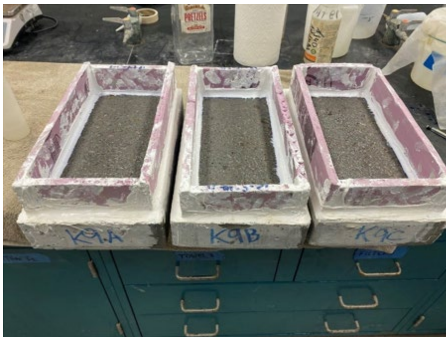
Figure 2.5: Scaling specimens with polystyrene foam dikes attached
