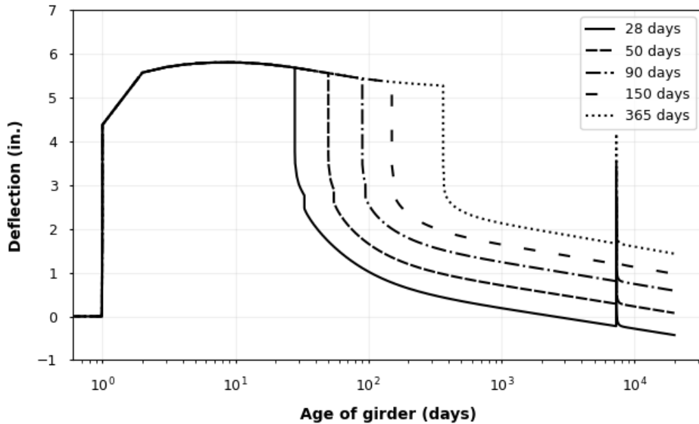
Figure 4.34: Midspan Girder Deflection by Age at Deck Placement
