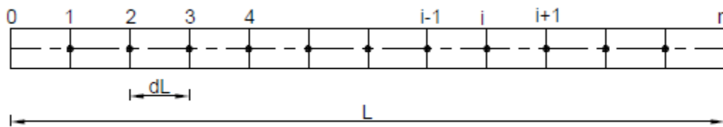
Figure 3.10: Division of Girder into Segments for Analysis
